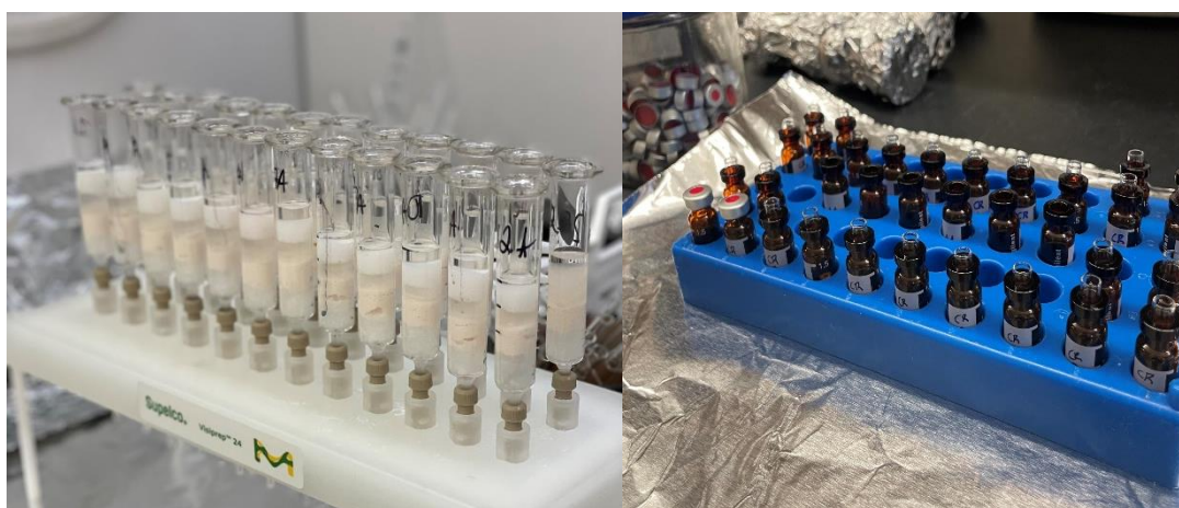
Figure 9. The photo on the left shows the cleaning process of the extractions and the photo on the right is of the final vials being readied for mass spectrometry.
